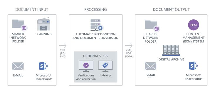
ABBYY FineReader Server receives document images from shared network folders, scanners, e-mails, and Microsoft® SharePoint® and automatically converts them into searchable digital formats using optical character recognition (OCR) technology. If needed, the user can manually correct text information and/or add metadata to the document. The resulting digitized files can be saved to any number of storage areas and/or delivered to other applications.
